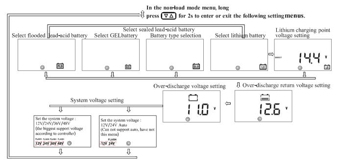
Battery Types, Charging Voltages (Lithium Battery), Over-Discharge Return and Over-Discharge Voltage Settings
